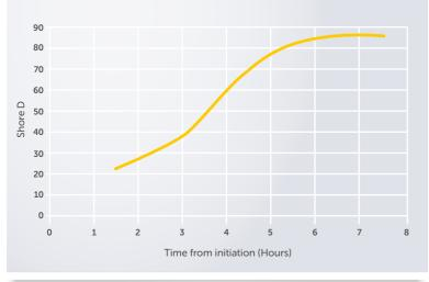
Crestapol® 1250LV -Typical Shore-D hardness development 2% Accelerator G, 2% Trigonox 239. Room temperature vacuum infusion processing. 2 ply 600T woven glass fabric laminate.
